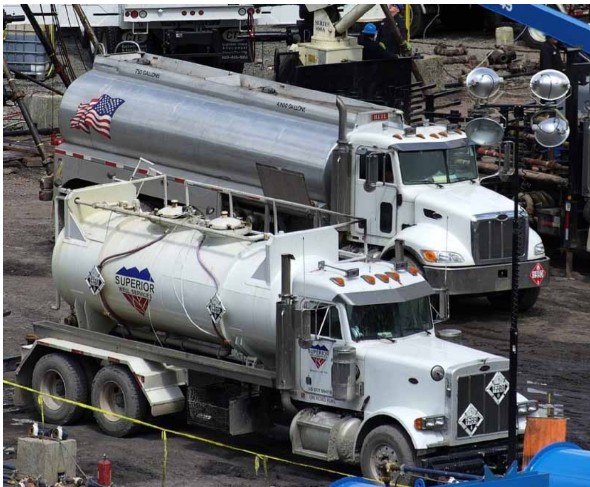
Photo 5.19 - Transport trucks for water (above) and hydraulic fracturing acid (HCl) (below)
