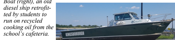
Boat (right), an old diesel ship retrofitted by students to run on recycled cooking oil from the school's cafeteria.
